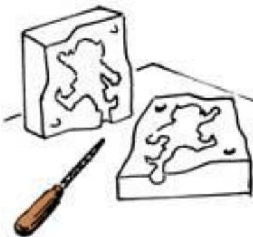
**Step 15:** At this time, check each half of the mold for any under-cuts that can be cut back. Let your mold dry out for 4 or 5 days depending on your weather conditions. NOW YOU HAVE A MOLD.
