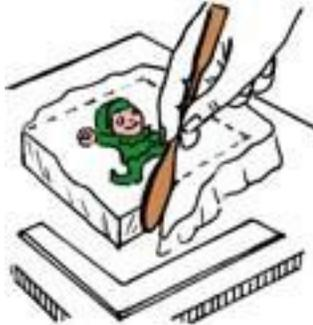
**Step 4:** Apply Parting Agent with a soft brush covering the entire surface. Dry your brush and pick up all excess Parting Agent, leaving a very slick surface on the object and parting line clay.
