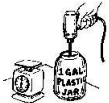
**Step 7:** Let the plaster soak for 3-5 minutes, then mix with your Drill Motor Mixer. Mix for about 1 1/2 minutes, then pour over boxed pattern. **Plaster should cover at least 1 inch over the highest point on the Model.**
